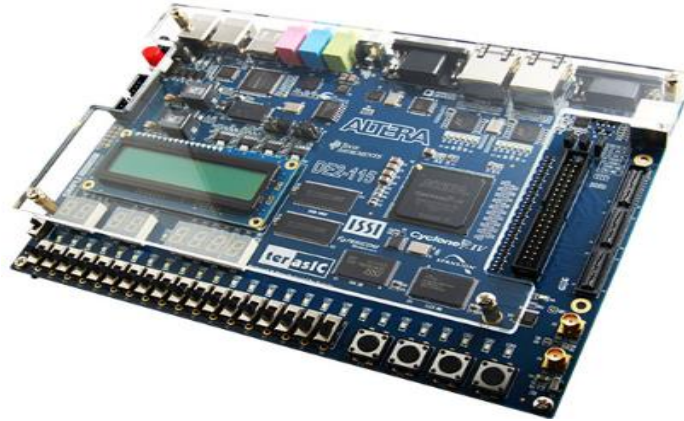
Figure 10: DE2-115 FPGA development system from Altera (INTEL)
